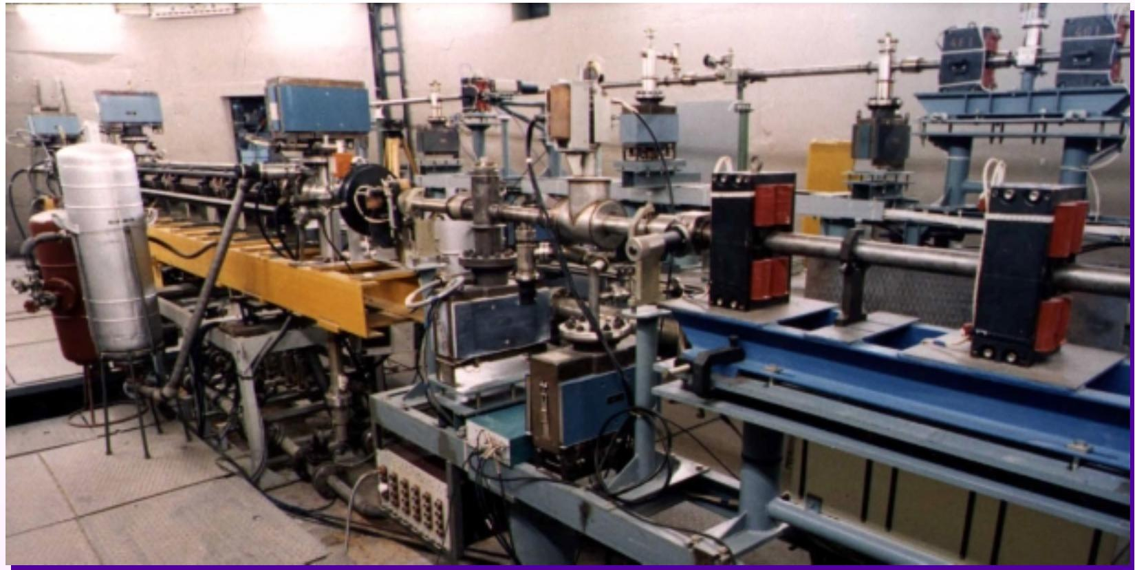
**Electrons are accelerated to an energy of 100 MeV**
