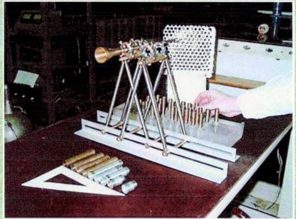
RF detector with the set of waveguide cut-off filters
