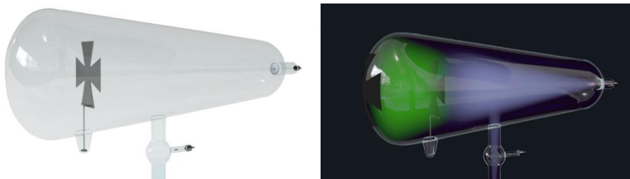
Fig. 1.1.1. Cathode rays cause fluorescence on the walls of the glass tube. A solid object placed in the path of the cathode rays casts a shadow on the wall of the tube across from the cathode
