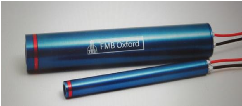
Fig. 5.5.51. Scintillation counter with Phi 30 and Phi 13 mm NaI(Tl) crystals
