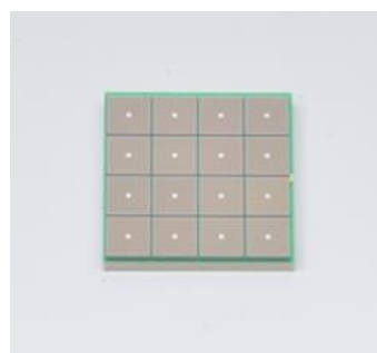
Fig. 5.5.31. A matrix of 16 SiPMs
