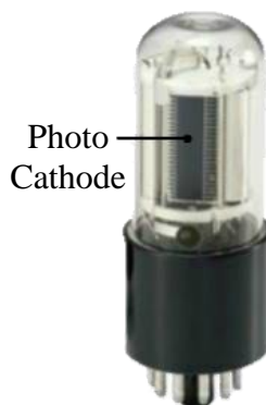
Fig. 5.5.18. A side-on PMT – Hamamatsu R928
