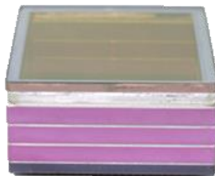
Fig. 5.5.49. A 144-channel HPD
