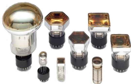
Fig. 5.5.15. A variety of head-on photomultipliers produced by Hamamatsu
