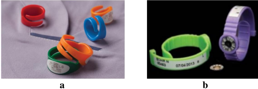
Fig. 5.4.3. Extremity TLDs designed as: a) rings; b) bracelets
