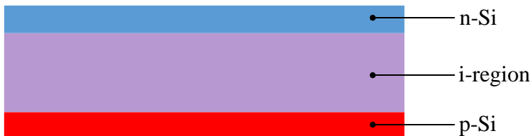
Fig. 5.3.10. Structure of a lithium-drifted silicon detector
