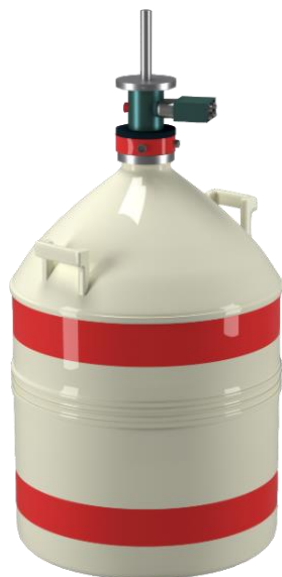
Fig. 5.3.11. A cryostat with the Si(Li) detector
