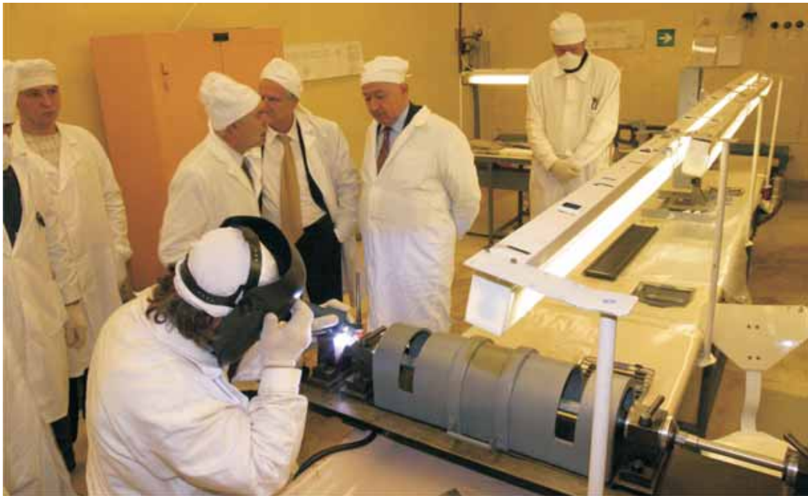
Frank Laboratory of Neutron Physics. The mounting of fuel elements into fuel assemblies for the IBR-2M reactor core
