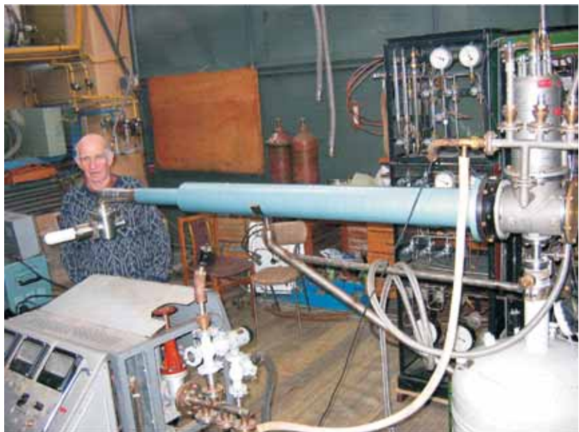
The liquid hydrogen target of the NIS setup and one of its authors V. F. Chumakov
