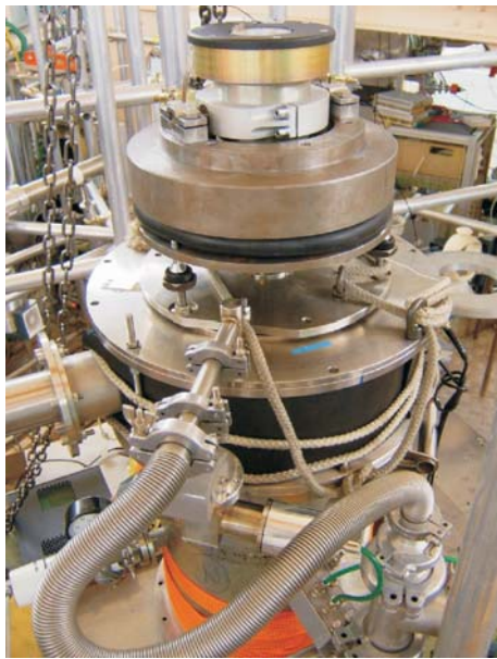
Fig. 2. Gravitational UCN spectrometer. An electro-magnet driver inducing harmonical motion to the sample is installed at the upper flange
