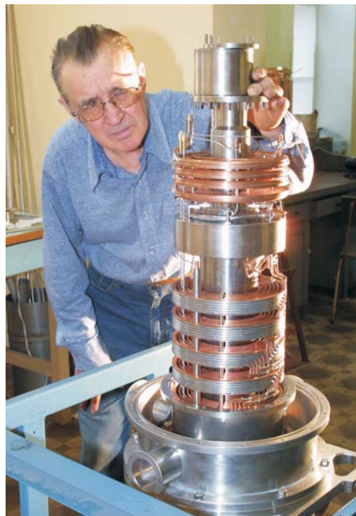
Laboratory of Nuclear Problems. The cryostat produced by JINR staff members for a new polarized target of Mainz University (Germany)
