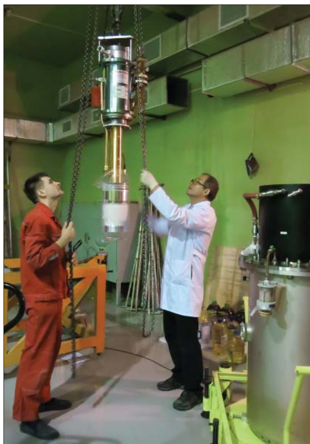
The Frank Laboratory of Neutron Physics. Assembling of new modulators for the IREN facility
