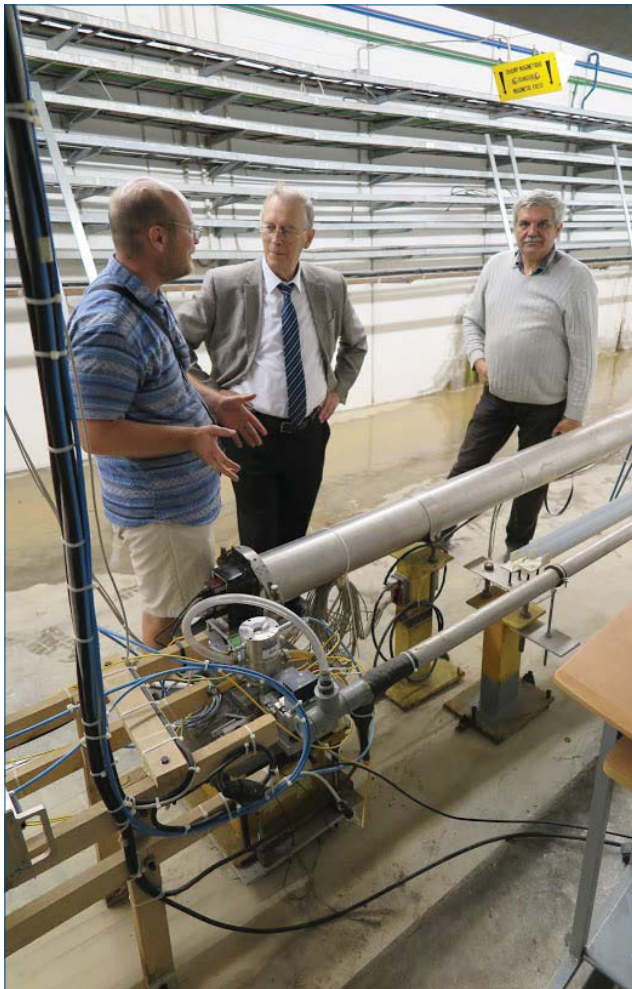
CERN (Geneva, Switzerland), June. JINR Director V. Matveev is shown the laser precision inclinometer developed by the JINR staff members
