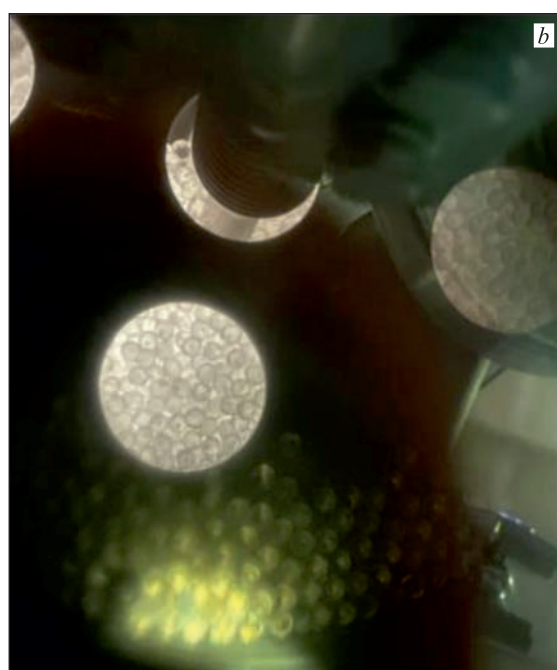
Modified dosing device with high unloading speed: a) the outer part of the cryostat; b) frozen beads during loading in real time
