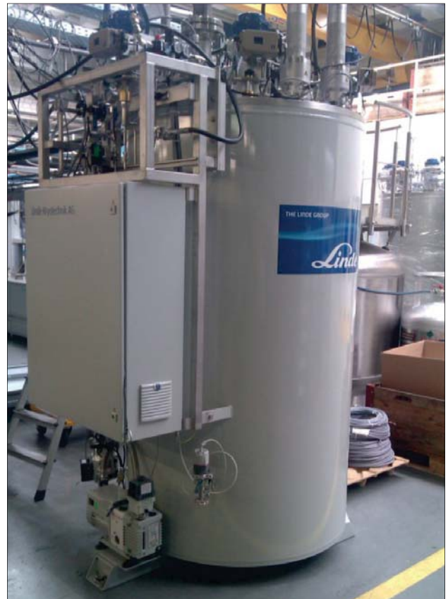
Helium cooling unit of KGU 1200/10
