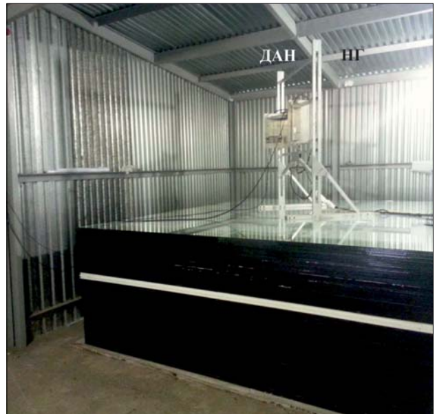
Planetary soil model with the DAN instrument and neutron generator (NG) above it
