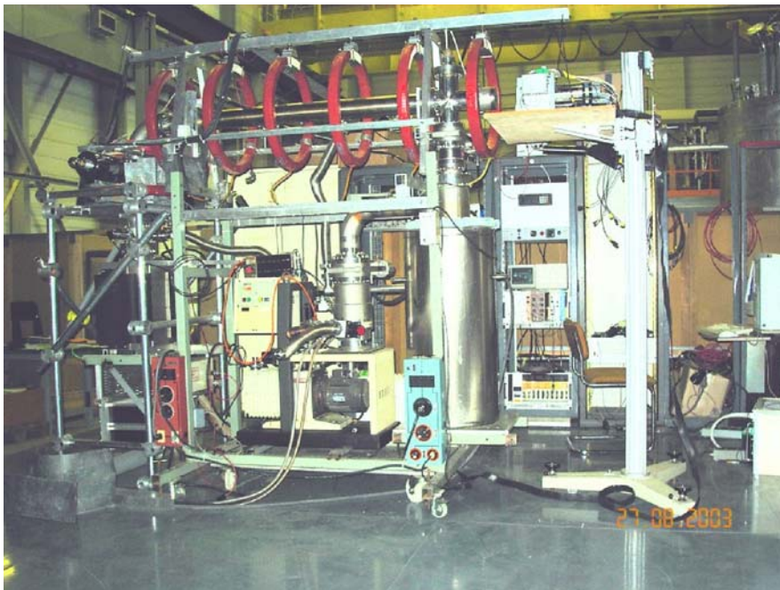
Fig. 8. Photograph of the ETH-INR slow-positron pulsed beam prototype
