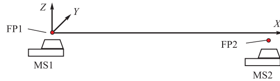
Fig. 18. A conventional reference frame of a local XYZ coordinate system. X axis: positive towards FP2, the second fiducial point in such a way that Y_{FP2} = 0.0 ; Y axis: perpendicular to X in such a way that the system is right-hand oriented; Z axis: perpendicular to the plane XY and positive to the top. Origin: FP1 defined as a fiducial point, X_{FP1} = 0.0 , Y_{FP1} = 0.0 , Z_{FP1} = 0.0
