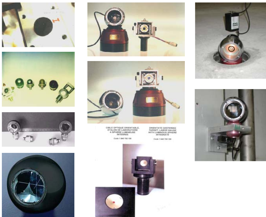
Fig. 24. Various types of targets on socket or specific adapter (CERN TS-SU-EM library)
