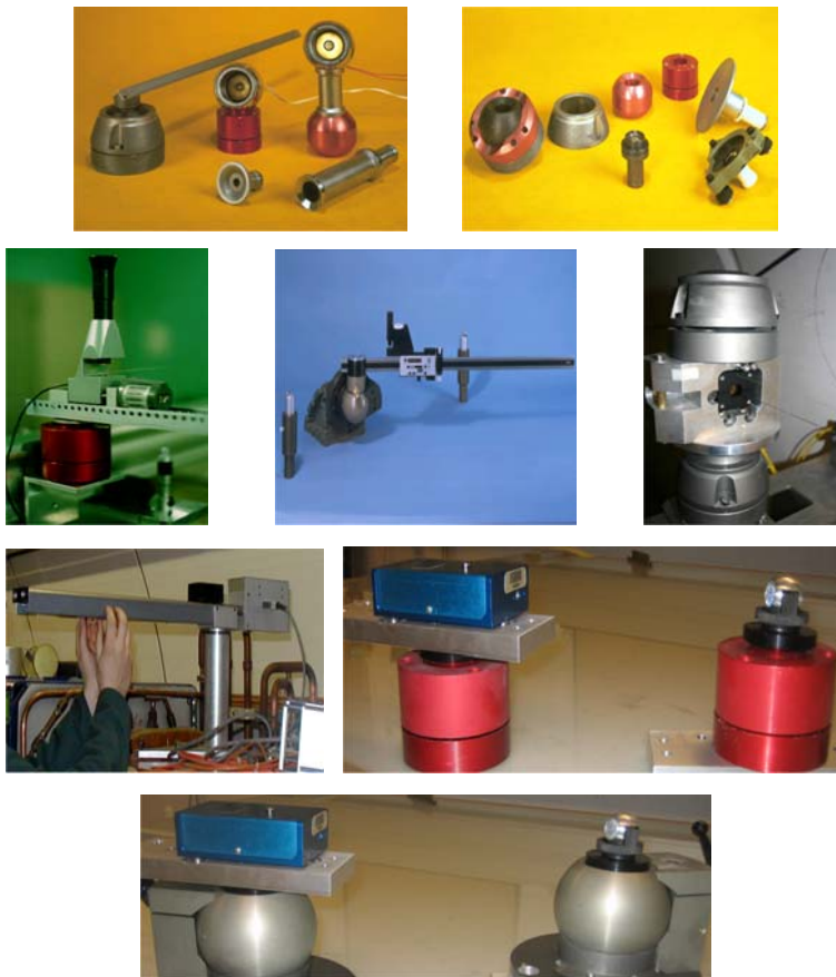
Fig. 26. Specific socket adaptations for various types of measures (CERN TS-SU-EM library)
