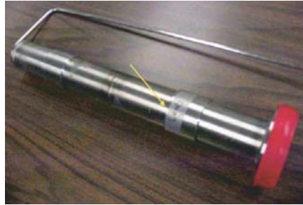
Fig. 35. Arrow points to the place where the leak occurred in tube 8A, which is the titanium–collar joint
