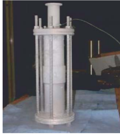
Fig. 27. Photo of a joint before the heating by the hot gun started
