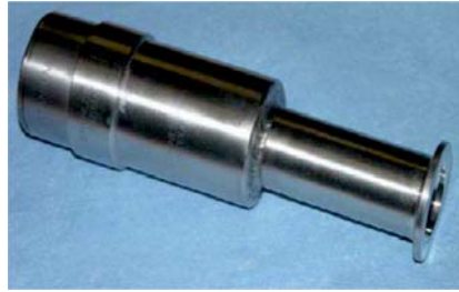
Fig. 21. The finished welded assembly
