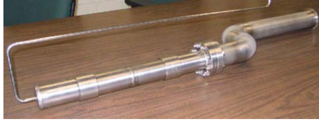
Fig. 32. Pair of tubes connected with their titanium ends ready for tests in the horizontal test system
