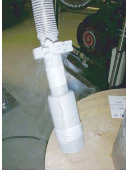
Fig. 22. Thermal cycling test with the Ti–SS transition sample having the welded components — cooled sample
