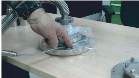
Fig. 43. Pumped-out assembly is placed in a plastic bag and the He gas is being blown in
