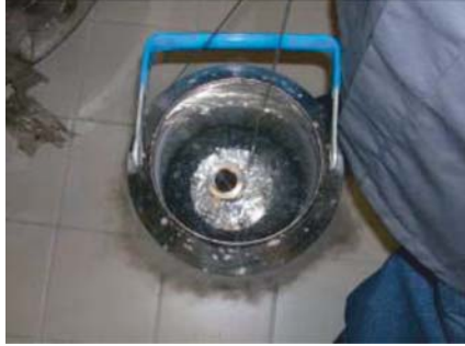
Fig. 26. Photo of a sample dipped in liquid nitrogen within the Dewar
