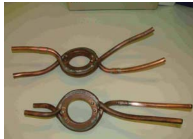
Fig. 29. Water-cooled copper heat sinks
