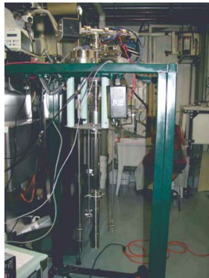
Fig. 34. Transition joint test article mounted on the top insert, prior to installation in the A0VTD
