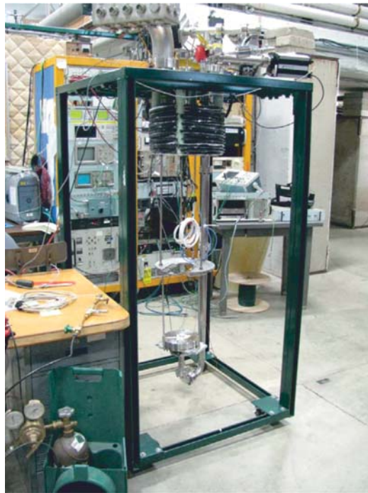
Fig. 46. Test article 2 ready for insertion into the VTD
