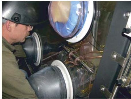
Fig. 28. Welding the titanium ends of the transition joint test article
