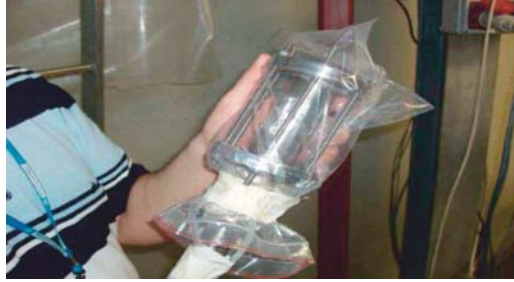
Fig. 16. The Ti–SS transition sample wrapped with a plastic bag for the leak test
