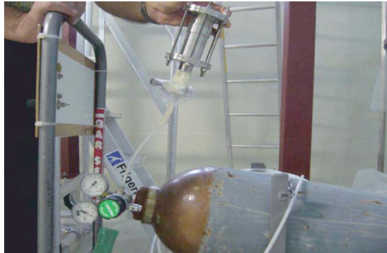
Fig. 19. The sample connected to the helium bottle and filled with gaseous helium up to a pressure of about 6 bar
