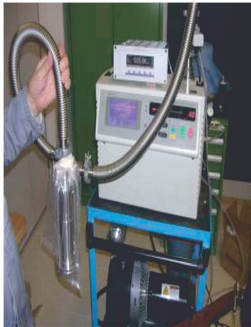
Fig. 25. The Ti–SS transition joint enclosed in a plastic bag for the He leak test measurements
