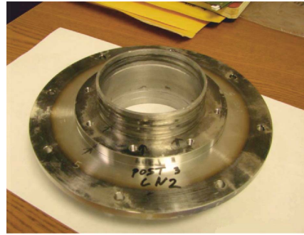
Fig. 45. Nb-SS transition joint with the identified leak points
