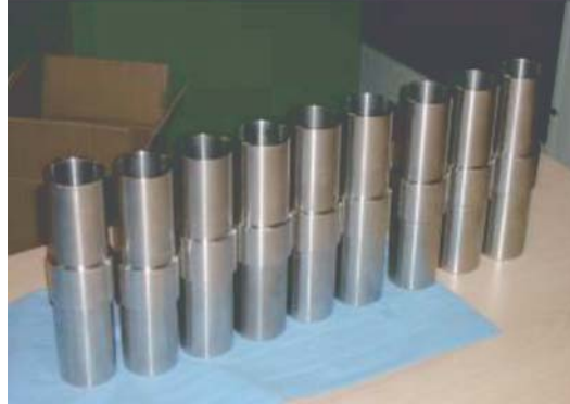
Fig. 24. Photo of the nine Ti-SS samples tested in Pisa
