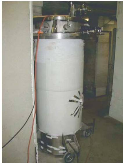
Fig. 33. A0 vertical test Dewar
