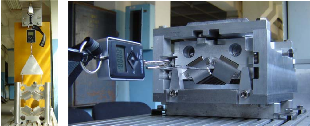
Fig. 5. Measurement of the vertical attraction force (left), measurement of longitudinal repulsive force (right)
