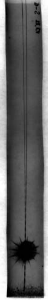
Fig. 7. The photo of the diffraction pattern, in the scale 1:1, produced by two tungsten wires. The radius of the cylindrical surface R = 140 mm. The maximal elongation from the central order is equal to 170 mm ( \theta > 1 rad)
