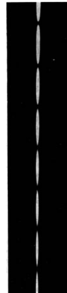
Fig. 2. Fragment of the diffraction pattern produced by the tungsten wire of the diameter \cong 26 \mu\text{m} . The distance between two successive minima is equal to about 4 mm on the real photo-negative
