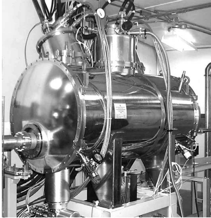
Fig. 1. Photo of 2 T 63-pole superconducting wiggler for Canadian Light Source
