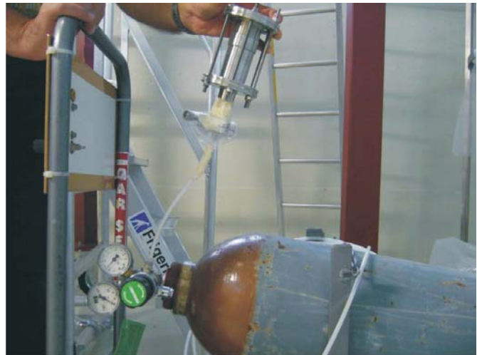
Fig. 9. The sample connected to the helium bottle and filled with gaseous helium up to a pressure of about 6 bar
