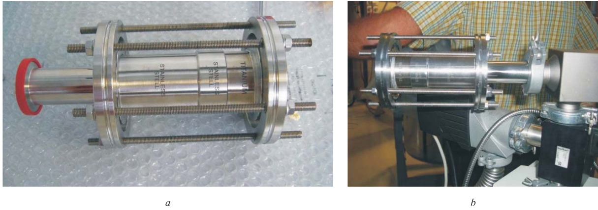
Fig. 4. Experimental set-up of the Ti-SS transition sample: a) to be tested; b) connected to the leak detector with a C-clamp
