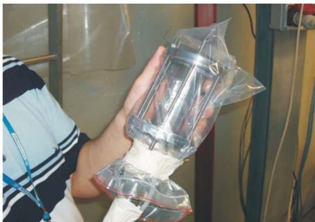
Fig. 5. The Ti-SS transition sample wrapped with a plastic bag for the leak test measurements
