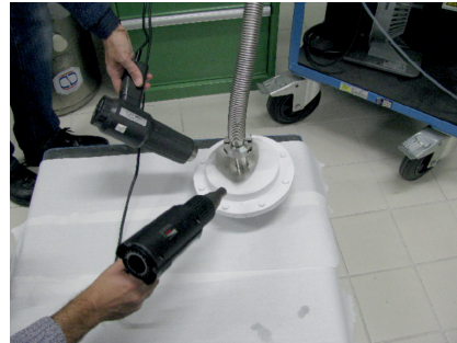
Fig. 14. Heating with heat guns
