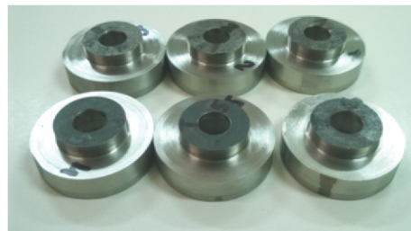
Fig. 10. The scheme of layer tear test and the general appearance of the samples
