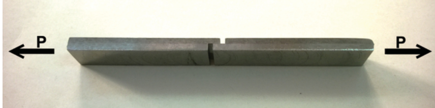
Fig. 11. The scheme of layer shear test
