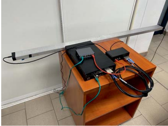
Fig. 1. MCORD system demonstrator with one scintillator
