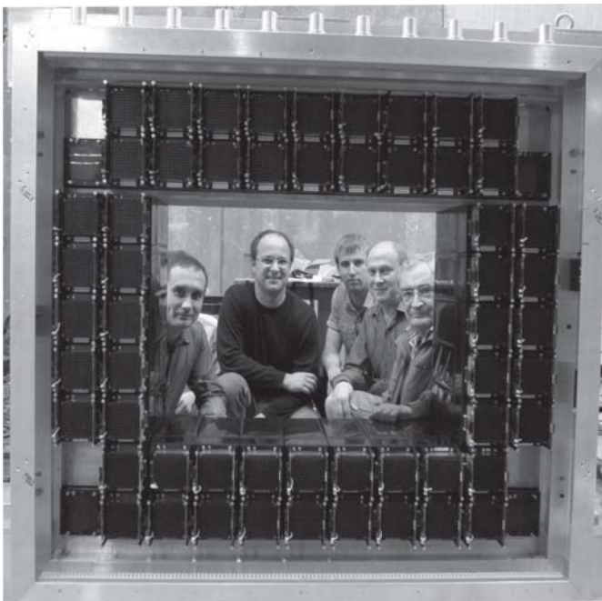
Dzhelepov Laboratory of Nuclear Problems. JINR team members during assembling of 56 ECAL0 modules for the DVCS tests at COMPASS-II (CERN)
