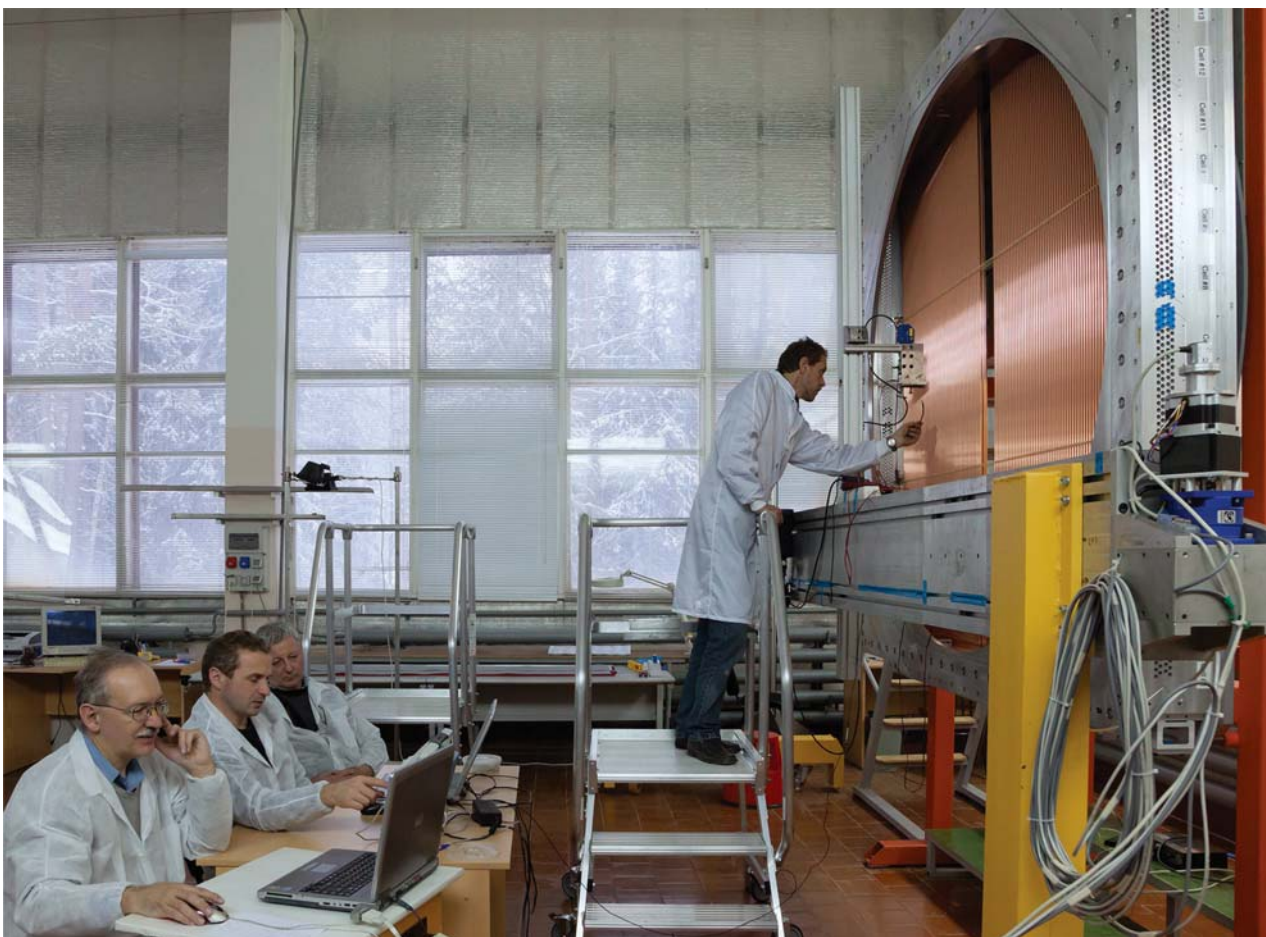
Veksler and Baldin Laboratory of High Energy Physics. Manufacture of full-scale modules of the straw detector for the NA62 experiment
