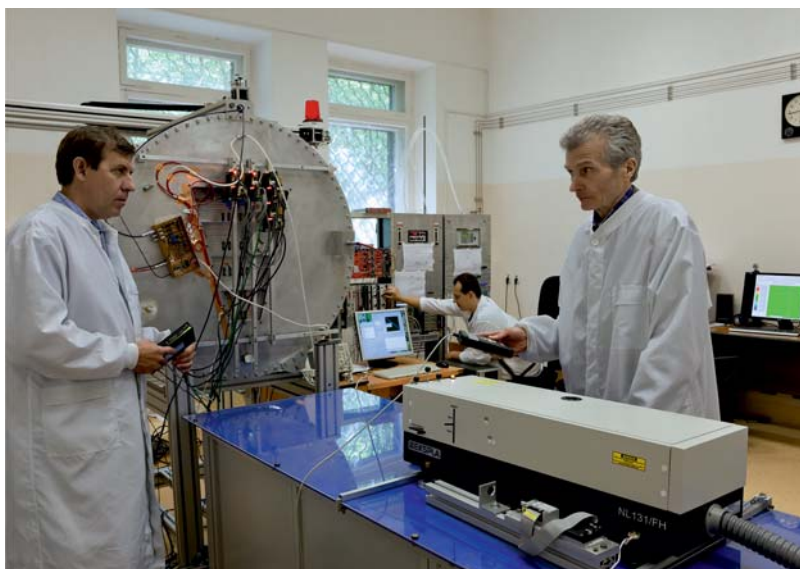
Veksler and Baldin Laboratory of High Energy Physics. A prototype of the time projection chamber TPC for the multi-purpose detector MPD for NICA
