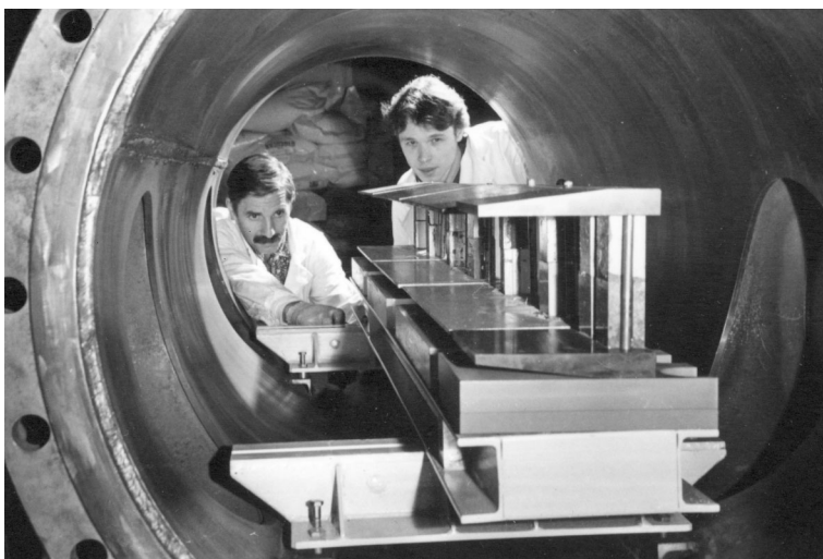
Frank Laboratory of Neutron Physics. Assembling of the magnet channel of the SPN-2 spectrometer
