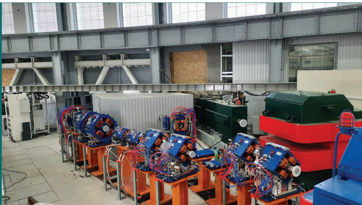
The Veksler and Baldin Laboratory of High Energy Physics. Beam transport channels in the applied research area
