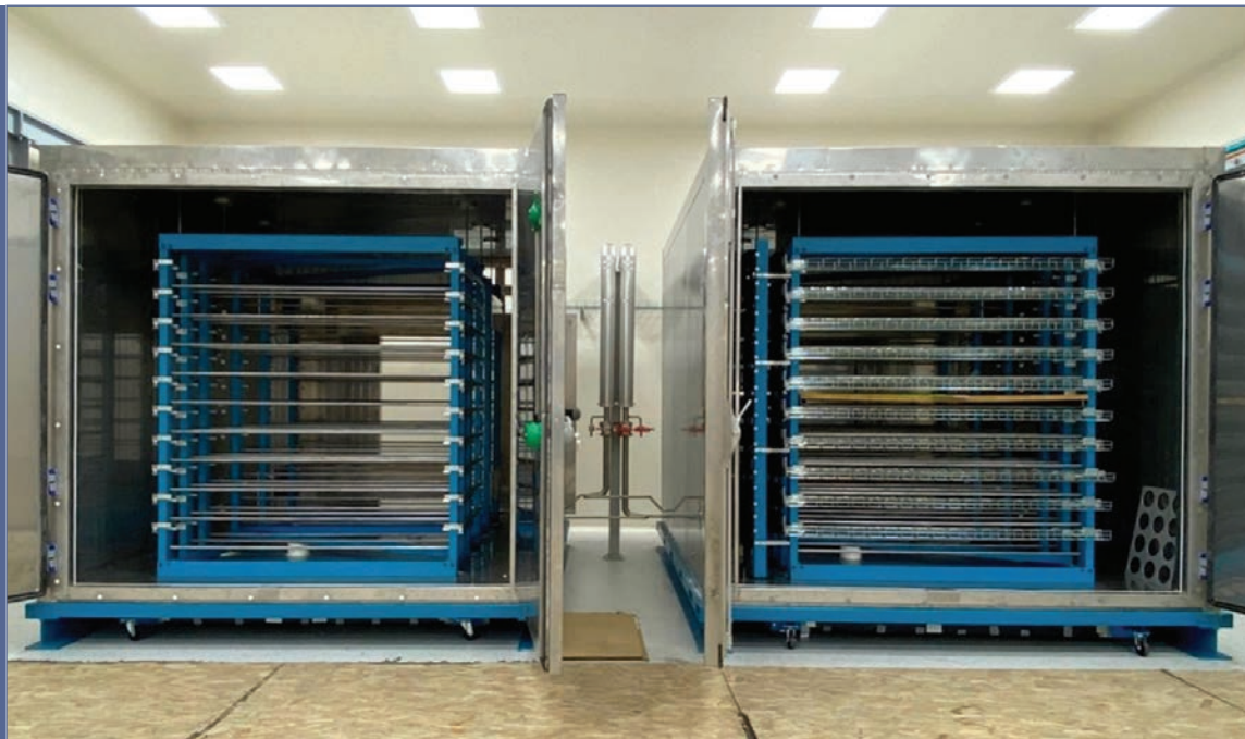
Thermally insulated chambers of the stand for testing cassettes of the high granularity calorimeter HGCAL, CMS
