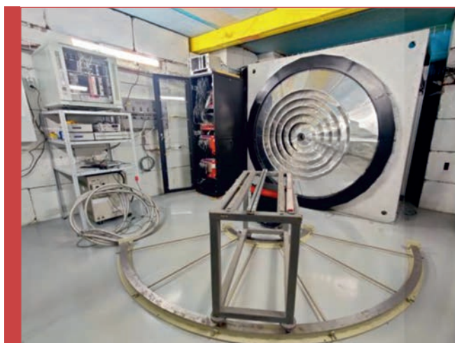
Left: Detector from the sample side, in the foreground — the mounted rotary platform for the 2D PSD detector and the sample environment modules, in the background — the backscattering detector and the data acquisition system. Right: Detector from the neutron guide side, with mounted and connected photomultipliers
