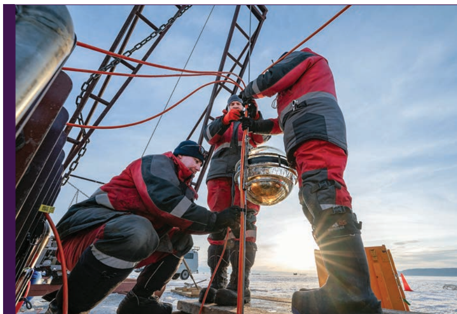
Lake Baikal, April. Installation of a garland of optical modules of the Baikal-GVD Neutrino Telescope
