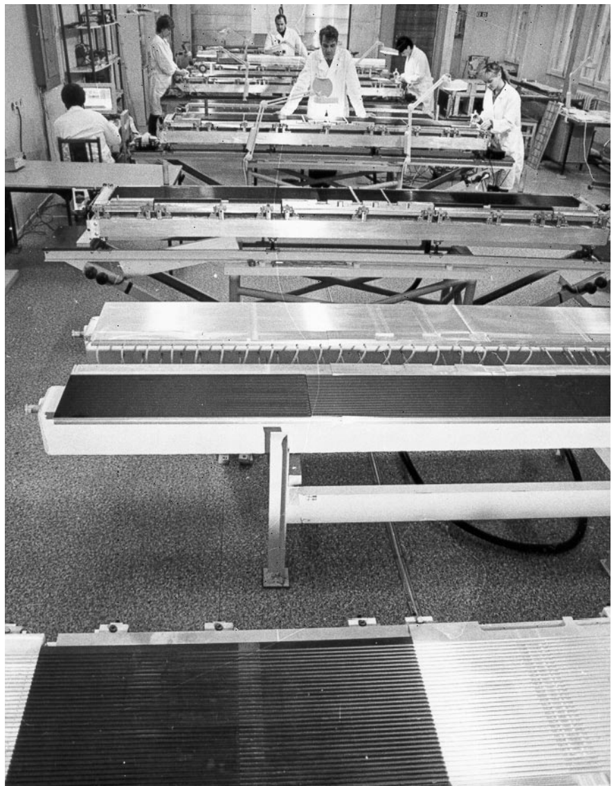
Laboratory of Particle Physics. Area for serial assembly of pokalon-C chamber modules for the HERA-B facility at DESY (Germany)
