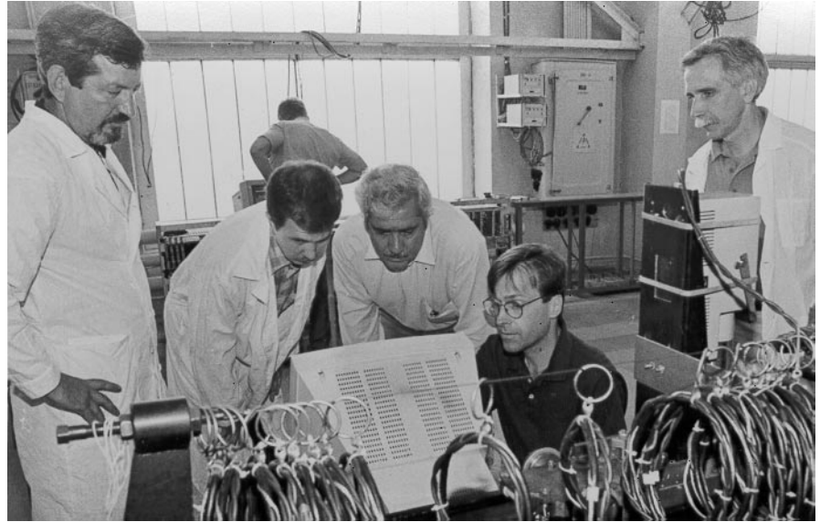
JINR Experimental Workshop. Area for testing mini-drift chambers purposed for physics research at the Tevatron in Fermilab (USA) within the D0 project
